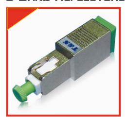
FBG ID Connector, with optical connector at on end, and optical adapter at the other end, is easy for fiber connector. When wavelength interrogator send certain ranged WDM signals to FBG ID Connector, the FBG will reflect certain wavelengths, so as to detect the fiber connection.
