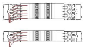
NOTE: The incoming of fibers on the left side of the support block must follow the paths indicated in the picture. In the same way mirror paths must be done in case of incoming of fibers on the right side.
