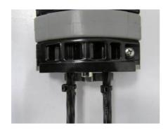
4.3.2.9 Fix the kit bracket to the subframe from the rear and loosen the Allen screws of the cable turrets Grease the outer silicon part of the cold sealing kit
