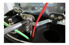
4.2.1.8 Clean the inlet and abrade its surface with abrasive tape.
