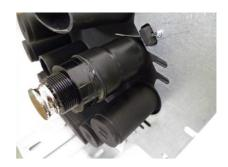
NOTE: The continuity plug has 9 numbered contacts. The G/V cable containing the mechanical core of the minicable or the ground cable of the STD cable must be welded to the contacts of the continuity plug.
