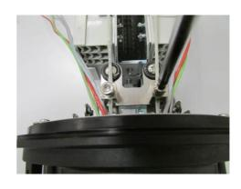
4.3.2.18 Free the metallic core of the cable (both the parts) contained in the VTR central core up to the cable holder tower
