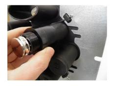
3.4.2 After the insertion of the plug the ground contacts must be protruded towards the internal part of the base.
