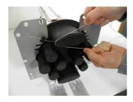
3.3.2 Circular inlet: place the steel wire for cutting on the inlet to be used and cut
