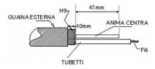
4.2.1.4 Fix the central core of the cable to the cable clamp of the kit OF0048
