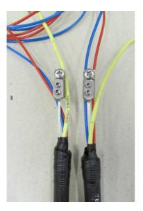
4.2.2.5 Fix the cable holders on the bracket included in the kit.
