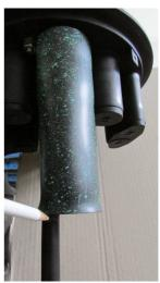
4.2.1.10 In correspondence of the mark, wind the cable with the Aluminium sheet making the marked line on the sheet match the mark on the cable
