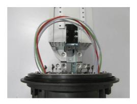
4.3.2.11 Insert the body of the kit inside the inlet up to the stop, inserting the fiberglass cores in the cable turrets and being careful not to damage the tubes
