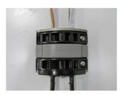
4.3.2.7 Re-insert and lightly tighten the Allen screw N.5 up to point 0 (position in which the compression of the gasket is zero)
