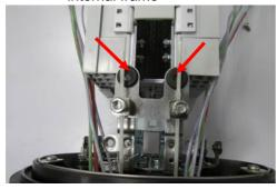
4.3.2.16 Tighten the previously removed cross head screws to fix the bracket to the frame
