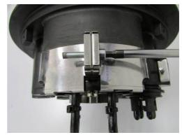
4.3.2.13 Take the upper bracket for core cable fixing and unscrew the two M4 hexagonal head screws
