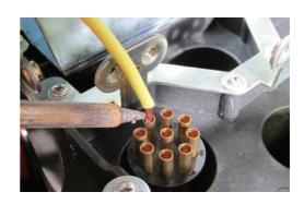
NOTE: cut the G/V cable at the right length depending on the position of the used inlet respecting to the inlet n° 12 of the continuity plug
