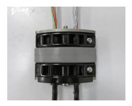
NOTE: make sure that the gasket is closed tightly on the cable
