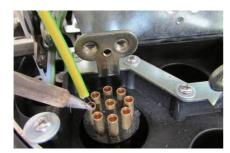
4.3.1.13 Proceed to the closing of the circular inlet screwing the Hexagonal head screw (n.3) doing 5 complete rounds (360°) from position 0 of the screw (position in which there is no crushing of the gasket)
