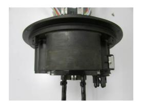
4.3.2.12 Slide the fixing jaw of the kit towards the inlet of the splice closure (with the Allen key facing the side of the two circular openings), get to the stop and tighten the Allen screw n.4 until the two parts are coupled
