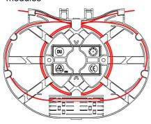
Example of arrangement internally on SF junction modules of single fibers jointed with heat shrinkable sheath.
