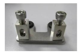
4.3.2.14 Insert the two parts of the central core of the cable in the two cable holder towers
