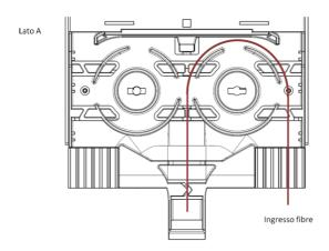
Example of transit of fibers from side A to side B with incoming fibers on the right of side A
