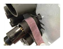
3.4.5 Insert the heat shrinking sleeve on the transition inlets/plug (surfaces previously cleaned and abraded).
