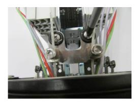
4.3.2.17 Tighten the M4 hexagonal head screws of the clamps to block the central core of the cable
