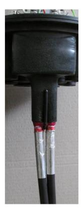
4.3 Loose tube minicables (cold sealing kit)
