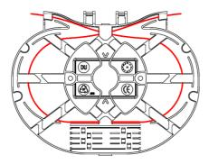
Example of arrangement of single continous fibers, single circuit for loose tubes cables, internally on SF junction modules
