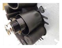
3.4.6 Shrink the heat-shrinkable sheath with thermal gun. After the shrinking the adhesive must be slightly outside from the edge of the sheath.
