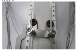
4.3.2.15 Slide the bracket towards the bottom up to align the fixation point to the internal frame
