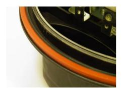
NOTA: the right side of the o-ring gasket is that where the round part goes in touch with the internal surface of the base, while its square corner looks towards outside.
