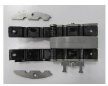
4.3.2.4 Pass the continuous tubes of the cable through the fixing jaw of the kit and slide it down along the cable so that it does not disturb the following operations
