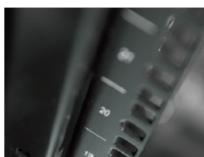
19" uprights numbered and adjustable in depth.
